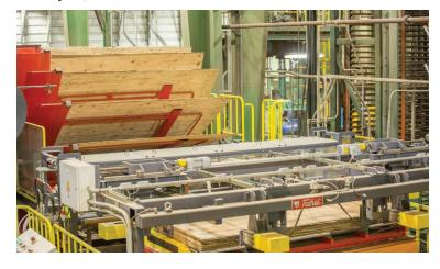
**LYONS, OR** - Freres Lumber Co. Inc. said it is the first U.S. manufacturer to install and operate the Taihei Horizontal Press Model P25-AB, a horizontal hot press for laminating plywood after the gluing and prepressing processes. The press was installed between Thanksgiving and Christmas and was fully operational on Dec. 17.
