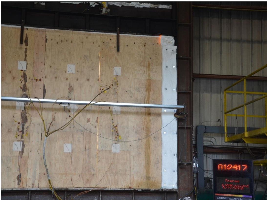
Figure B-10. Exposed Face 1 h 24 min, Flaming Visible through Joint.
