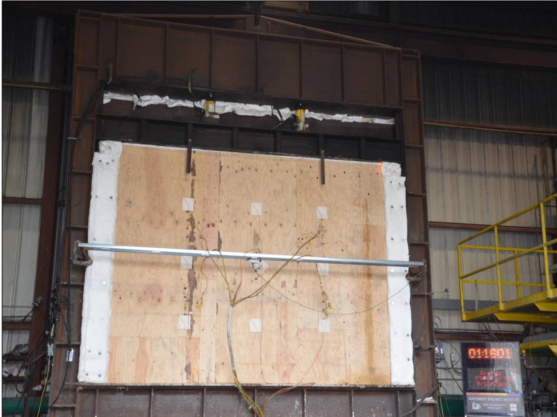
Figure B-9. Exposed Face 1 h 16 min, Flaming Visible on Top Right.
