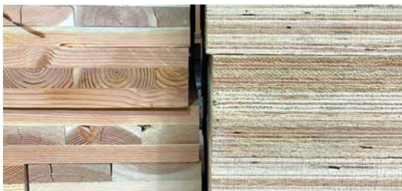
LUMBER-BASED CLT VS. VENEER-BASED CLT
