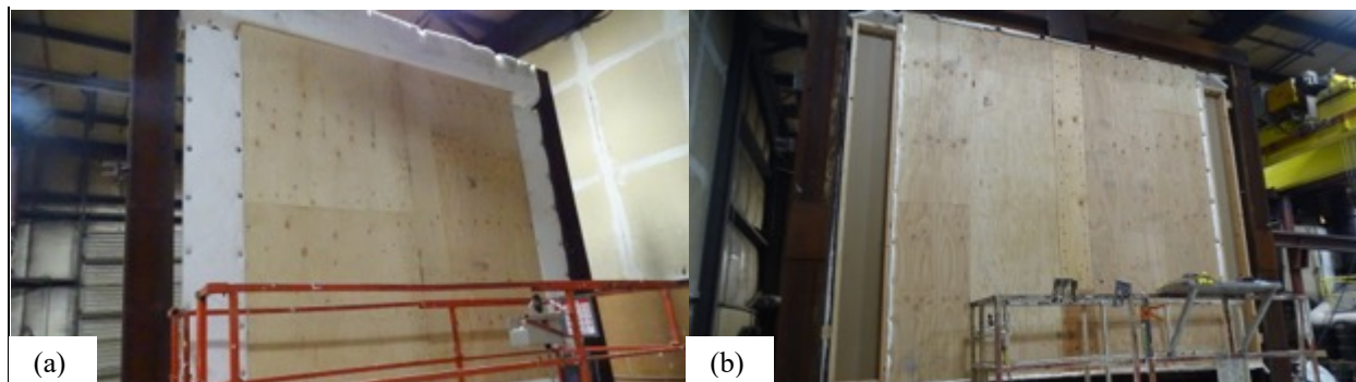
Figure 1. Representative MPP panels showing joined assembly (a) exposed side and (b) unexposed side with spline.
