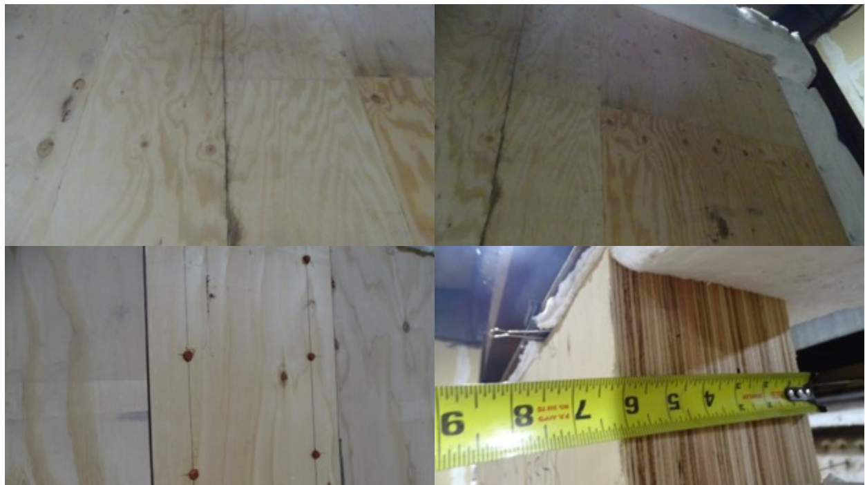
Figure A 2. Construction showing (a) exposed joint, (b) exposed side, (c) spline fasteners, and (d) thickness.
