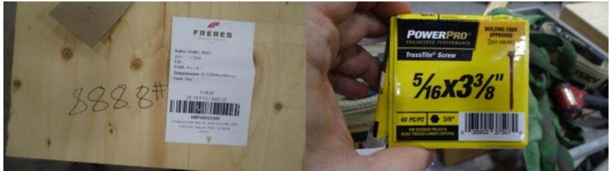
Figure A 1. Component identification showing (a) panel and (b) spline fasteners.
